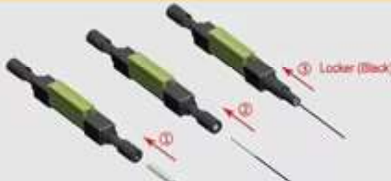
5. Install the sleeve, then carefully insert the fiber to the end and push forward the locker to lock the \Phi 0.25\text{mm} fiber.
