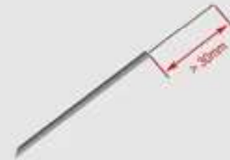
6. Use the miller pliers to strip 0.9 fiber coating.
