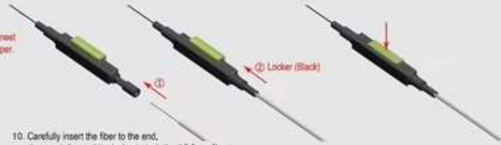
11. Press the side cover, complete the assembly.
