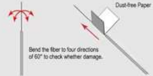
7. Check the fiber and clean the fiber.
